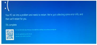
If you are running Windows 10, please make sure that any **Quick Shutdown** options are disabled – these features can cause a BSOD when the SSD7101A-1/SSD7204/SSD7104/SSD7120/SSD6540/SSD6540M/SSD7180/SSD7184/SSD7140 is installed into or removed from your motherboard. BSODs can be avoided by **completely powering off** your system.
